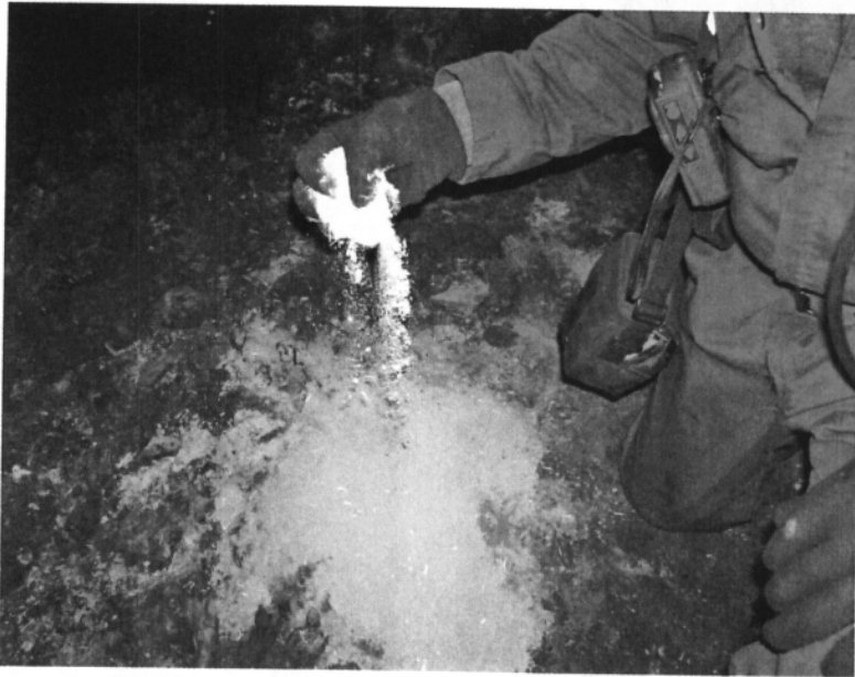
The forces of the explosion completely destroyed the Omega Block seal. Fine powder and dust was all that remained of most of the seal material.
